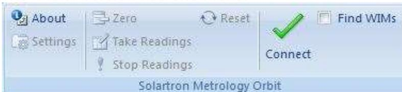
The functionality is the same but we no longer have the concept of a 'Link'. The user clicks on the Connect button which causes the application to search for available Orbit networks and modules.
