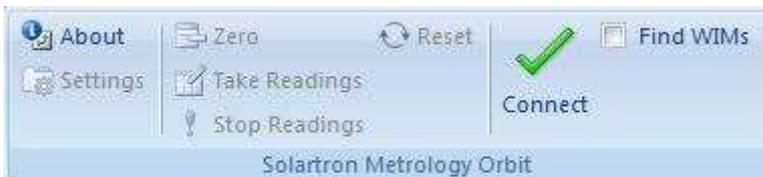
The main difference is that they have a textual description and the Connect button acts as a toggle to switch between connect and disconnect.
